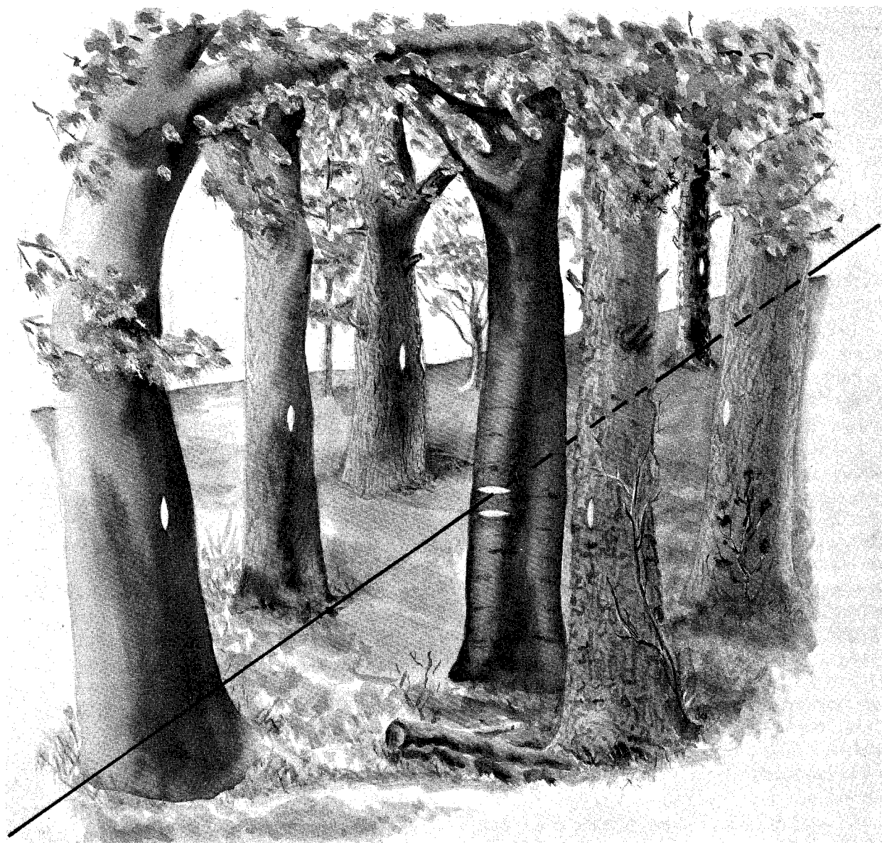
FIGURE 63.—Marking a line through timber.
